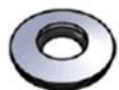
Sealing A soft neoprene washer bonded to a metal backing. Used to seal out air/water or dampen noise and vibration.
