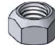
Prevailing Torque Lock A non-reversible lock nut used for high temperature applications.
